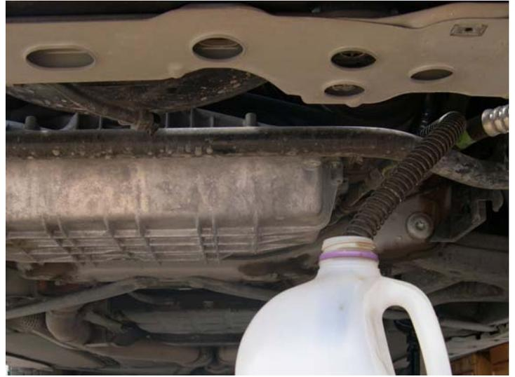
Now, you will have to make a decision. You can drain the transmission pan first, yielding about 3 quarts, or you can pump some fluid out, leaving a low enough level in the pan to remove it without draining it. Personally, I prefer the latter because it eliminates the possibility of having a stripped or leaking drain plug later. I look at this as "if it ain't broke, don't fix it."
