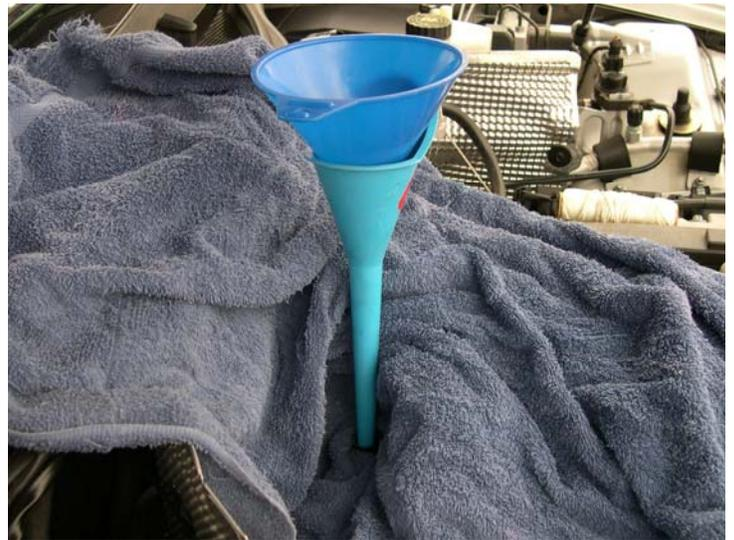
Pour the appropriate amount of new transmission fluid in via the funnel arrangement, taking care to pour slowly. If you pour fluid in faster than the small tube can carry it away, it won't back up in the funnel; rather, it will pour out of the top of the fill tube. The shop towels will absorb small amounts, but larger overflows will only soil your car and your driveway or garage, not to mention wasting expensive new transmission fluid.
